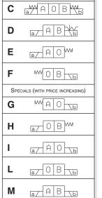
• Mounting type D is only for valves with detent
