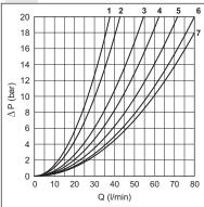
The diagram at the side shows the pressure drop curves for spools during normal usage. The fluid used is a mineral oil with a viscosity of 46 mm<sup>2</sup>/s at 40°C; the tests have been carried out at a fluid temperature of 40°C. For higher flow rates than those in the diagram, the losses will be those expressed by the following formula:
